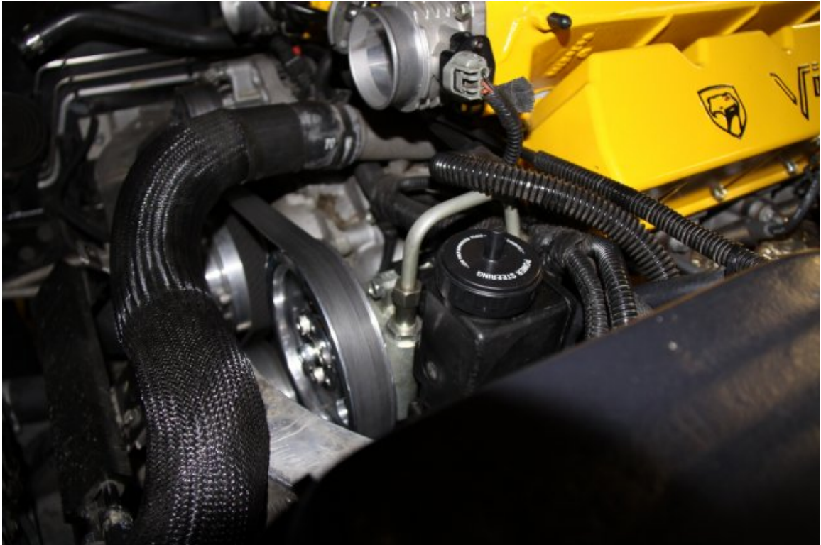
Photo #7 (Installed Pulley)
