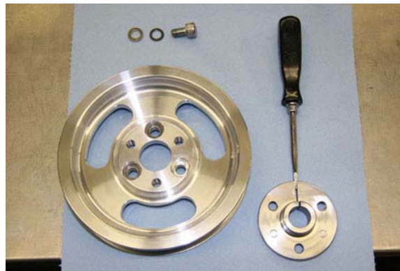
Photo #4 (Using small screwdriver to spread hub slot)
