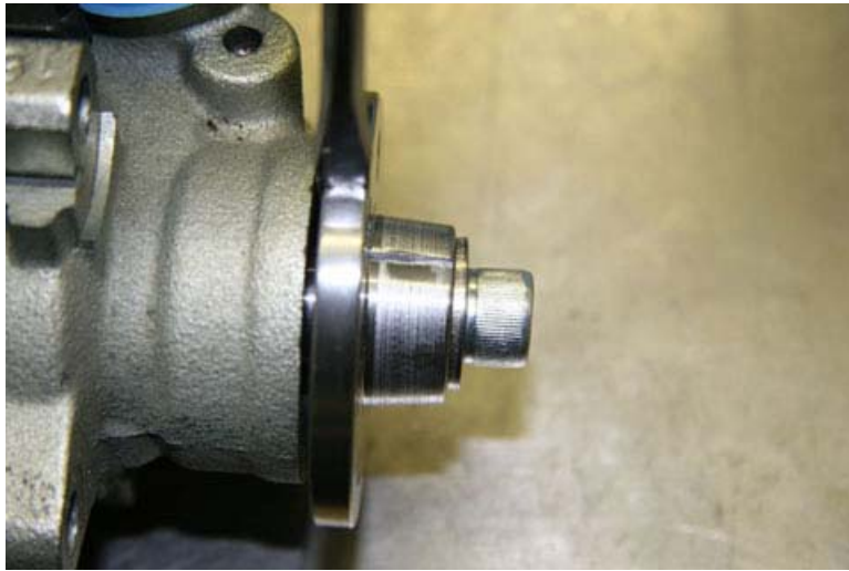
Photo #5 (Hub alignment with pump shaft and Housing)
