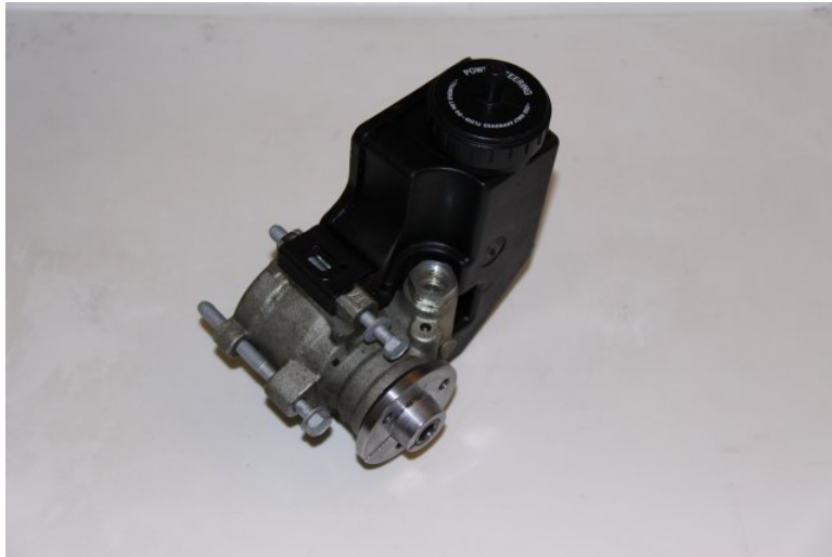
Photo #6 (Pump Mounting Bolts installed into Housing)
